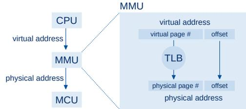
Figure 3.1: Diagram of the address translation process.
